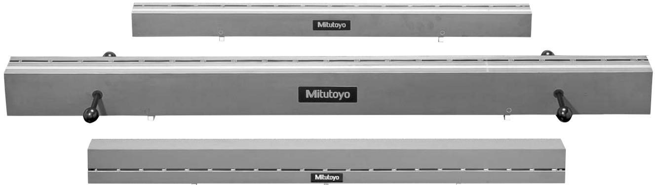
CERA Straight master is a master gage used for the straightness inspection of each axis movement such as a CMM, machine tool, semiconductor related equipment and form measuring machine. An alminaceramic material is adopted to achieve the significant weight reduction compared with the conventional masters made from a stone or iron. Double faced type is laping the double face which can be used for straightness in horizontal and vertical as a reference square.
