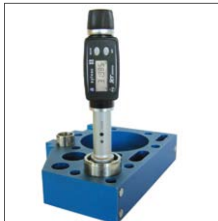
Measuring with ratchet XTD system
