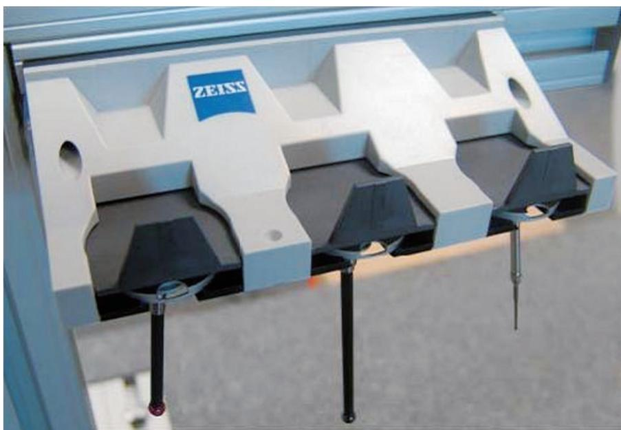
Stylus storage for VAST XXT fitted to the frame behind the table
