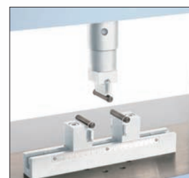
3-point bending test of plastic specimen
