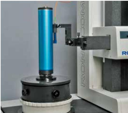
Sample of roundness measurement using a non-contact detector (option)
