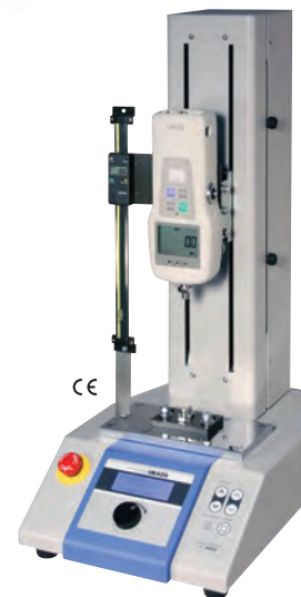
MX2-550-S with optional digital distance meter
