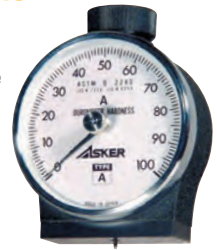
Model X with optional peak indicator Accuracy \pm .75 point
