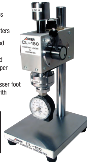
CL-150 Constant Load Stand Durometer and attachments sold separately
