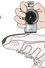
Super EX with optional peak indicator Accuracy \pm 1 point
