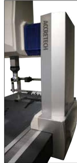
New developed covers are adopted for the X-axis guide and Y-axis carriage. Protecting the guide and carriage with covers reduces the impact of temperature changes, which enables to expanding the temperature range for guarantee accuracy of XYZAX AXCEL. The X-axis guide cover also prevents contaminants from attaching to the X-axis guide.
