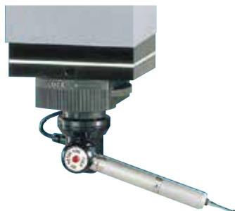
PH1 is a manual positioning probe head that allows positioning at the horizontal surface rotation angle of  $360^\circ$  ( $15^\circ$  pitch) and vertical surface rotation angle of  $\pm 115^\circ$ .
