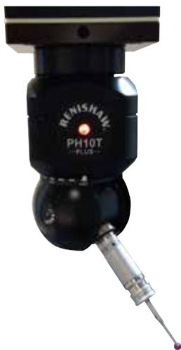
PH10T PLUS is a motorized indexing probe head whose horizontal surface rotation angle is  $\pm 180^\circ$  and whose vertical surface rotation angle is  $0$  to  $\pm 105^\circ$ . It allows positioning at a pitch of  $7.5^\circ$  in both directions.
