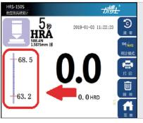
By setting the upper and lower limits of hardness alarm, the user can automatically pop up the pop-up window to indicate whether the user can save and print the test results
