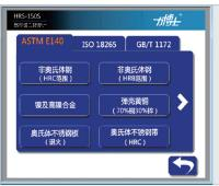
System integration—ASTM-E140-12be 、ISO-18265-2013、GB/T1172 three hardness conversion standards, automatic hardness conversion, no need to waste time to query cumbersome hardness comparison table
