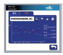
System built-in single point, multi-point mode, and multi-point mode provides hardness distribution curve data analysis function, automatically calculate the maximum, minimum, average value, easy for users to analyze the test data
