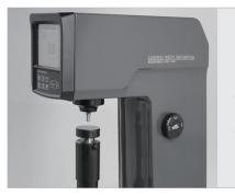
To control the loading, loading and unloading of the test force by means of a motor to eliminate the error
