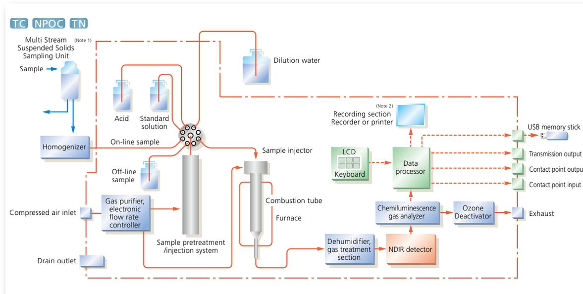
Note 1) For the sampling section, select the multi-stream suspended solids sampling unit, the single stream suspended solids sampling unit, the backwash strainer sampling unit or the sample stream kit (option).
