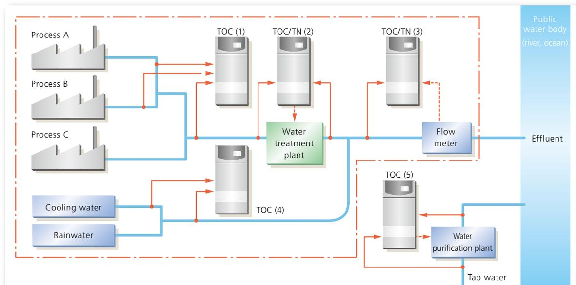
TOC (1) Monitoring of TOC values discharged from each process (three-flow-line switching)
