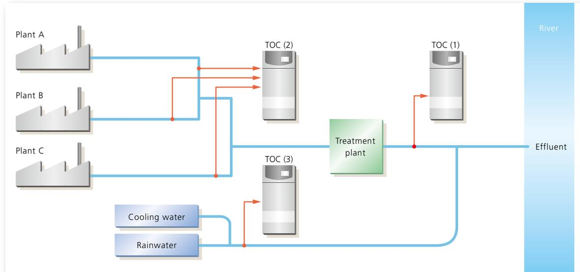
TOC (1) Prevents water pollution accidents through rapid detection of abnormal effluent.
